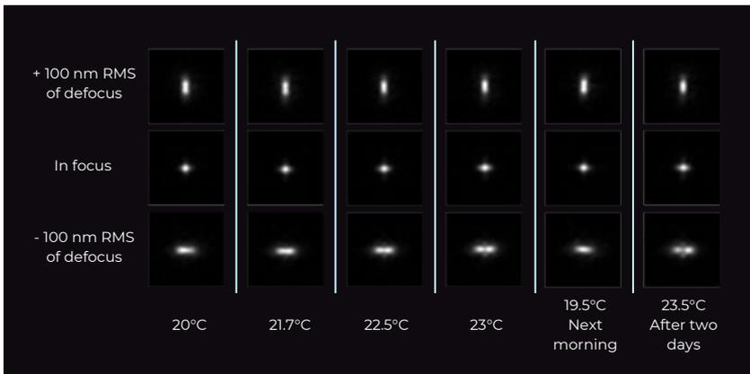
Example images of the diffraction-limited fluorescent bead at different ambient temperatures without stabilization module inside MicAO.
