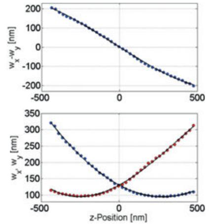
High lateral separation of astigmatic PSF along the whole Z range (up).
